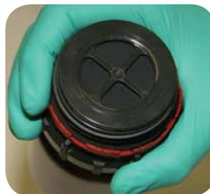
To get the best results from the septum, we recommend you use 18 to 21 gauge needles and puncture in a clock face pattern to avoid piercing the septum in the same place.
